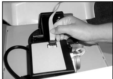
Figure 14: Connect the Ribbon Cable
