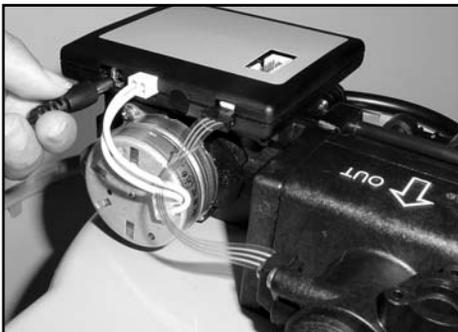
Figure 13: Connect Transformer Power Cord
