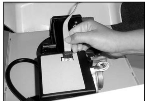
Figure 14: Connect the Ribbon Cable
