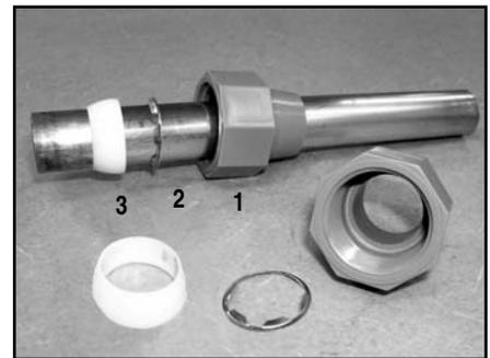
**Figure 5: Qest Fitting Assembly**
