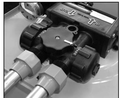
Figure 9: Bypass Position (Appliance shown with optional bypass.)
