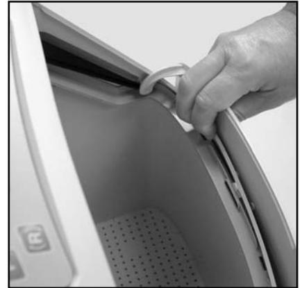
Figure 4: Remove Valve Cover
